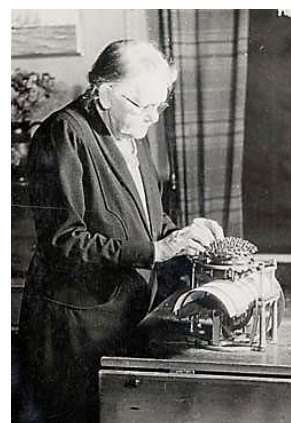
Left: A "writing ball typist". This writing ball from 1875 was rather high and should therefore be placed on a relatively low table in order to have a good typing position. Centre: Malling-Hansen's invention underwent continuous improvements, and can be found in a variety of versions. Presumably, old "balls" were disassembled and mounted on newer models. This is the model that was developed by mechanic August Lyngbye in 1885. Photo: Dieter Eberwein. Right: The publications for the writing ball claimed that it could be used by anybody, even persons suffering from trembling hands.
