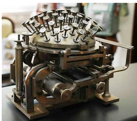
Left: A "writing ball typist". This writing ball from 1875 was rather high and should therefore be placed on a relatively low table in order to have a good typing position. Centre: Malling-Hansen's invention underwent continuous improvements, and can be found in a variety of versions. Presumably, old "balls" were disassembled and mounted on newer models. This is the model that was developed by mechanic August Lyngbye in 1885. Photo: Dieter Eberwein. Right: The publications for the writing ball claimed that it could be used by anybody, even persons suffering from trembling hands.
