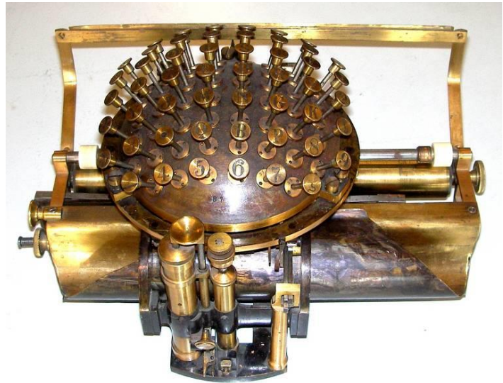
Left: The well known tall model of the writing ball, now with a color ribbon. It was ready in time for the World Exhibition in Paris in 1878, and was awarded with a gold medal. Copyright: Uwe Breker. Right: The last writing ball model also had paper platen and was equipped to type on large scale paper formats. It was developed by August Lyngbye who received a first prize medal at the Great Nordic exhibition in Copenhagen in 1888. Photo: Sverre Avnskog.
