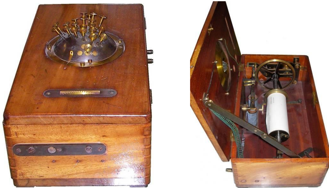
Two specimens of the first official model of the writing ball that was built into a wooden box still exist. This one is photographed in The Museum for science and technology in Elsinore. Photo: Sverre Avnskog
